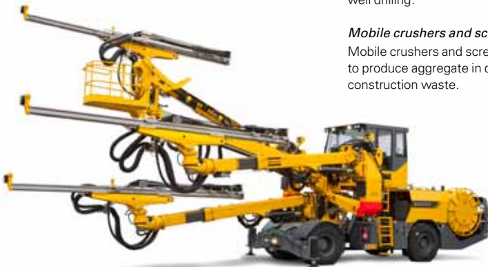
Underground drilling rig for tunnelling
